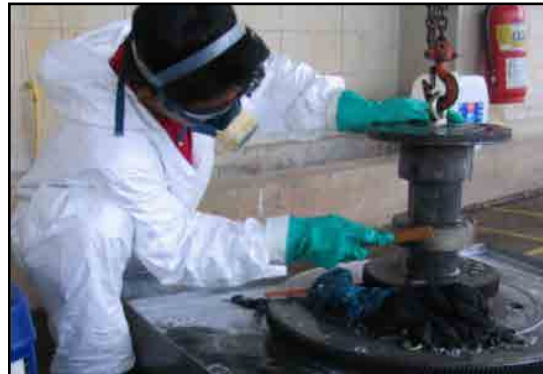
Cleaning corroded spare part with 338 Super Rust Remover.
