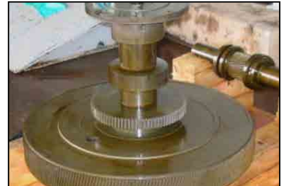
Cleaned spare part protected with a preventative coating of 740 Heavy Duty Rust Guard.
